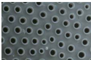
Figure 2a. Surface detail: Celpure diatom (96–98% SiO 2 ).
