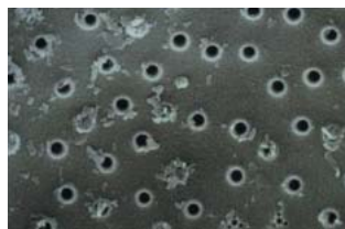
Figure 2b. Surface detail: conventional diatom (86–93% SiO 2 ).
