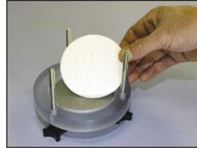
3. Place one gasket below and one on top of the cylindrical filter body.
