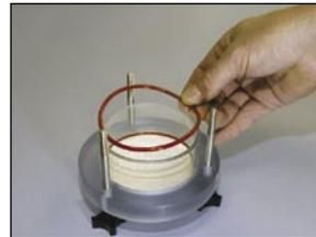
4. Place the top of the housing on the body and tighten the wing nuts. (Finger tightening is sufficient.)
