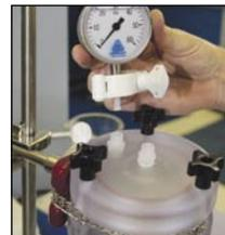
6. Insert the tube-end luer lock fittings on the inlet and outlet tubing and clamp. Secure inlet and outlet tubing to the filter via luer lock fittings.
