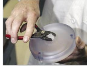
2. Insert bolts into the bottom of the housing. Place the metal septum support into the bottom of the housing. Place the septum (*i.e.*, depth filter) on the septum support.
