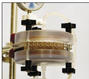
Figure 3a. This 50-cm<sup>2</sup>, 3-cm tall filter housing may be ordered from [www.ertelsop.com](http://www.ertelsop.com) (part # LAB 50P). Accessories are listed at the back of this document (Table 5).
