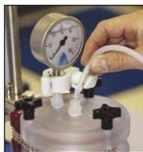
7. Fill the filter (using the pump) with a process-compatible solution. Fill from the bottom, allowing the air to rise to the top of the housing where it is vacated. All air pockets should be removed. Check for leaks and re-tighten the housing bolts as necessary. (Finger tightening is sufficient.)
